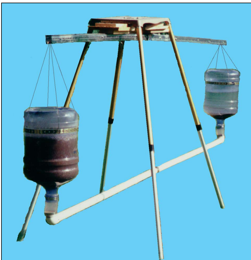
Figure 103: Liquefaction Demonstration. When the wooden blocks at the top of the horizontal beam are removed, the beam can rock like a teeter-totter. As the far end of the beam is tipped up, water flows from the far tank down through the pipe and up into the near tank, which holds a mixture of sediments. Once liquefaction begins, the sediments become mushy, their volume swells slightly, sedimentary particles fall or rise relative to each other, sorting themselves into layers, each having particles with similar size, shape, color and density. Buried objects with the density of plants and dead animals float up through the mushy sediments— until they reach a liquefaction lens . The same would happen to plants and animals buried during the flood.
