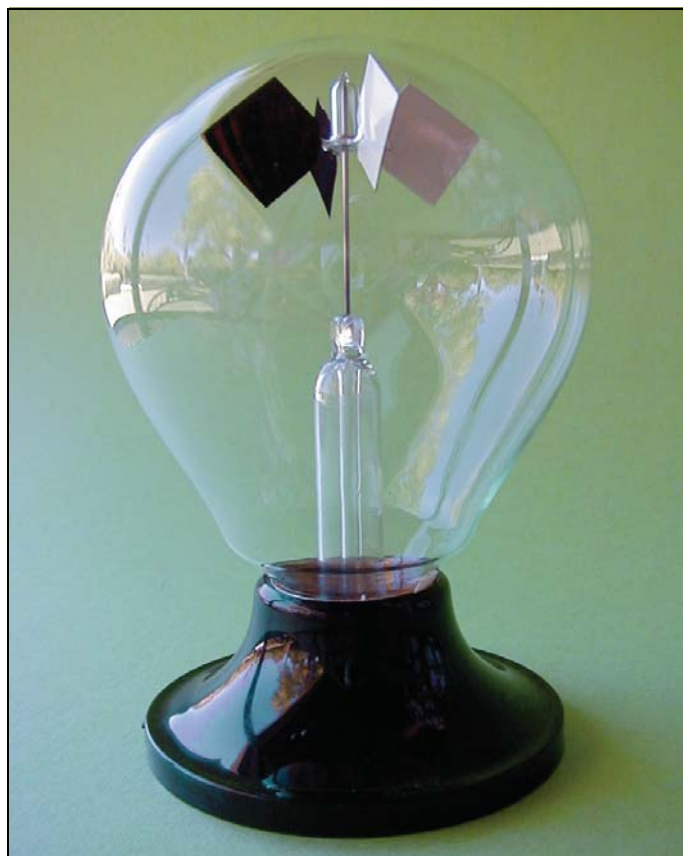
Figure 182: The Radiometer Effect. This well-known novelty, called a radiometer , demonstrates the unusual thrust that pushed asteroids into their present orbits. Sunlight warms the dark side of each vane more than the light side. A partial vacuum exists inside the bulb, so gas molecules travel relatively long distances before striking other molecules. On average, gas molecules bounce off the hotter, black side with greater velocity and momentum than off the colder, white side. This turns the vanes away from the dark side. 16
