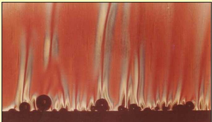
Figure 212: Thermocapillarity. Boiling removes heat from a hot solid by several powerful mechanisms. In one process, the surface tension surrounding a growing bubble propels the hot liquid away from the hot solid, so cooler liquid can circulate in and cool the solid. If cooler liquid is also flowing parallel to and beyond the hot, thermal boundary layer next to the solid, as it would have been with water flowing in vertical channels throughout the crust during and shortly after the flood, the tops of the growing bubbles would have been even cooler. Therefore, the surface tension at the tops of the bubbles would have been stronger yet, so heat removal by jetting would have been even more powerful.
