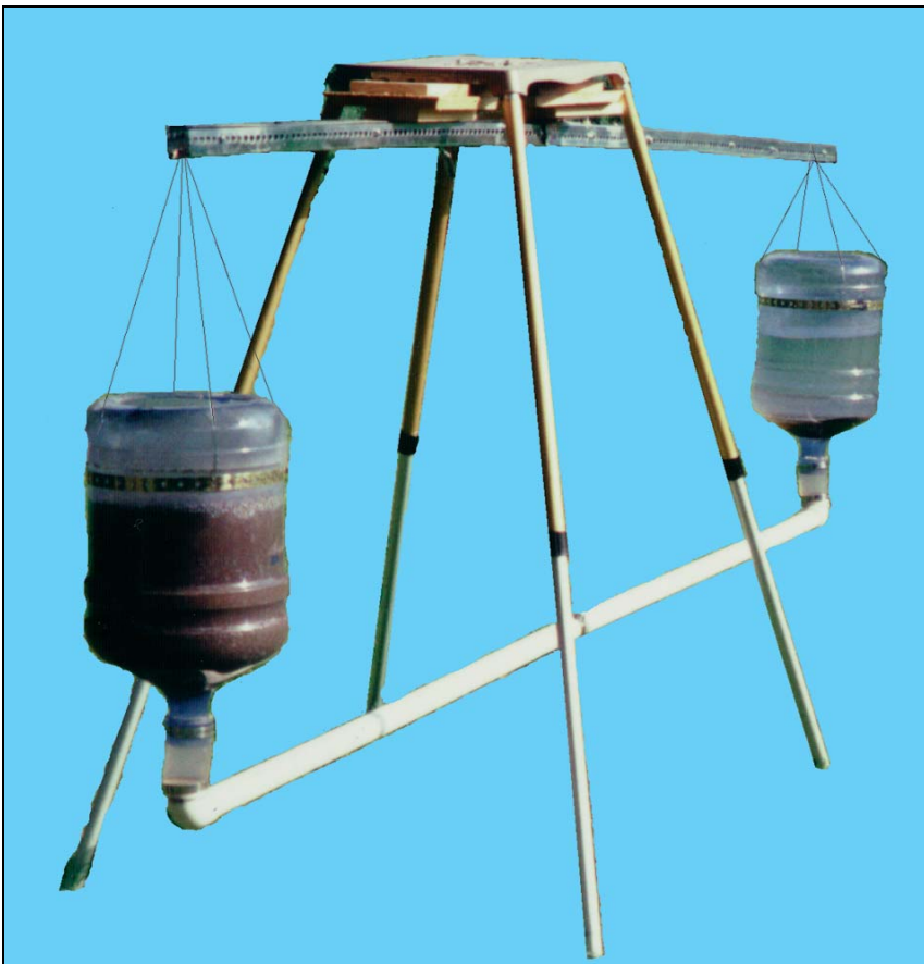
Figure 32: Liquefaction Demonstration. When the wooden blocks at the top of the horizontal beam are removed, the beam can rock like a teeter-totter. As the far end of the beam is tipped up, water flows from the far tank down through the pipe and up into the near tank, which holds a mixture of sediments. Once liquefaction begins, the sediments become mushy, their volume swells slightly, sedimentary particles fall or rise relative to each other, sorting themselves into layers, each having particles with similar size, shape, color and density. Buried objects with the density of plants and dead animals float up through the mushy sediments— until they reach a liquefaction lens . The same would happen to plants and animals buried during the flood.
