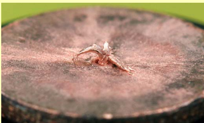
Figure 170: Ruptured Electrode. This disk (0.02 of an inch in diameter) is a slice of one of the thousands of electrodes that ruptured when a self-focused, relativistic electron beam pinched into a 630,000,000°F “hot dot” that was only 4 billionths of an inch in diameter. The focused heat was enough to melt a piece of rock a few millimeters in diameter. [See “Chondrules” on page 412.] Decay fragments and new chemical elements were splattered onto an accumulating screen for later analysis by a mass spectrometer.
