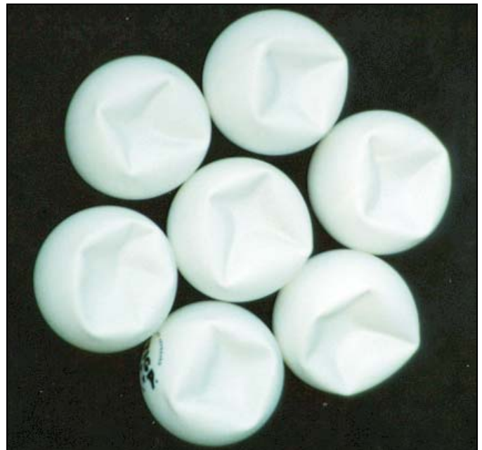
Figure 97: Deforming a Sphere Inward. When the hard outer shell of a ping-pong ball is depressed on one side, it deforms in an arc-and-cusp pattern. Materials always deform in a way that minimizes the energy required.
