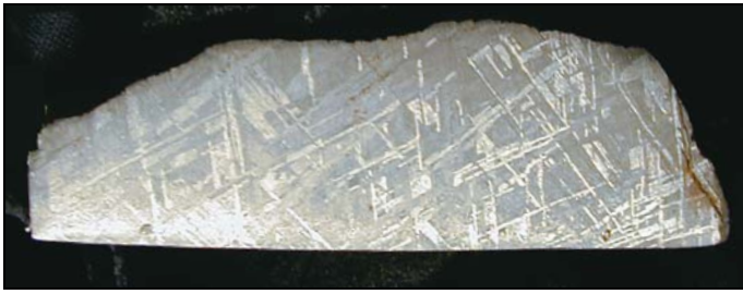
Figure 149: Hot Meteorites. Most iron-nickel meteorites display Widmanstätten patterns. That is, if an iron-nickel meteorite is cut and its face is polished and then etched with acid, the surface has the strange crisscross pattern shown above. This shows that temperatures throughout those meteorites exceeded 1,300°F. 20 Why were so many meteoroids, drifting in cold space, at one time so uniformly hot?
